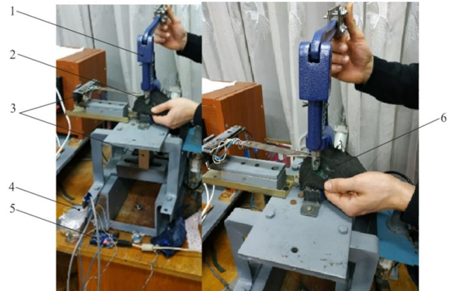
Figure 9 Experimental installation for the research of materials resistance at destruction with a wedge-shaped blade: 1 - cutting press; 2 - working organs (punch and stand); 3 - strain gauge; 4 - amplifier; 5 - analog-digital converter; 6 - material sample
