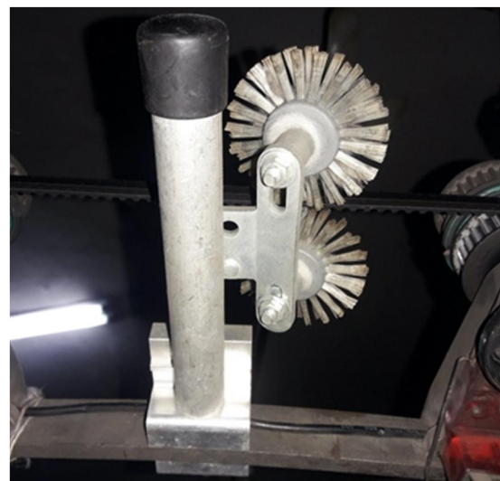
Figure 9 Single brush-shelf for circular knitting machine
