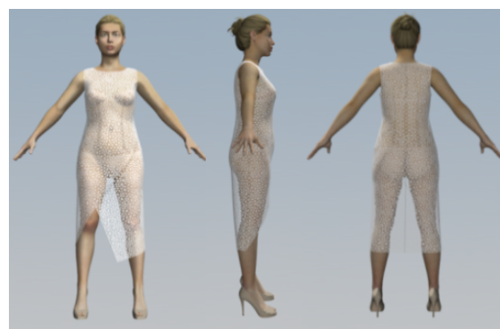
Figure 7 Virtual model of the dress in PDS Julivi to assess static compliance of mesh model
