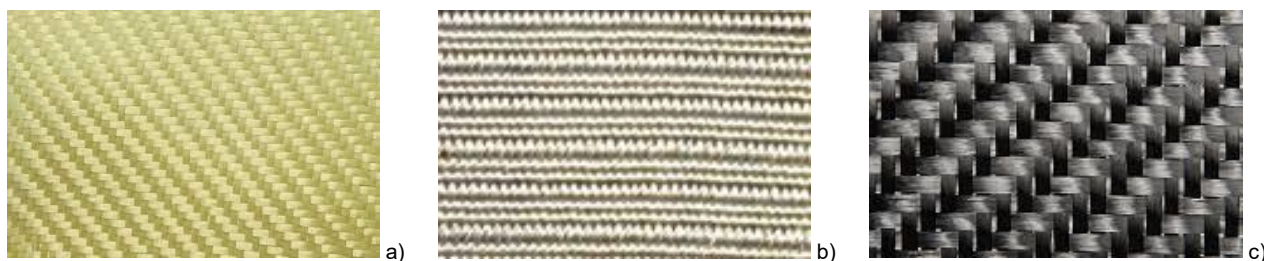
Figure 1 Industrial fabrics: a) Kevlar from para-aramid multifilament yarns 44 tex; b) Nomex from meta-aramid multifilament yarns 40 tex; c) fabric from carbon multifilament yarns 30 tex
