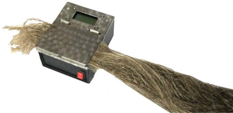
Figure 3. Placement of the sample in the measuring chamber of the device DDCIFF-1.
