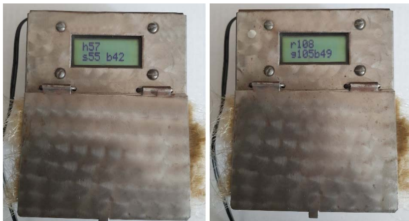
Figure 4. The digital display will show the color coordinates in HSB format, and if necessary, using the control panel, you can display the digital color coordinates in RGB format.
