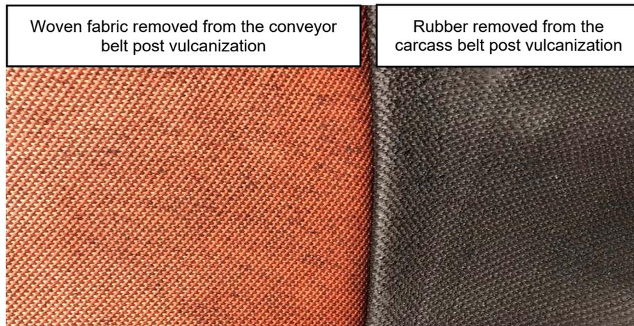
Figure 1. Woven fabric removed from conveyor belt reinforcement [1].
