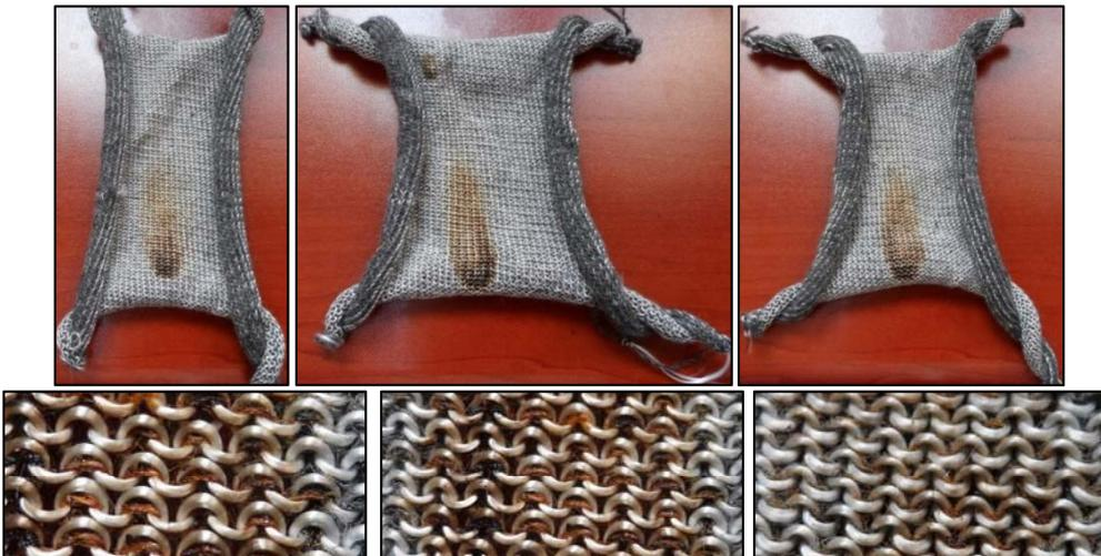
Figure 9. The photos of the burned WA/GG hybrid fabric knitted at 4 cam setting.
