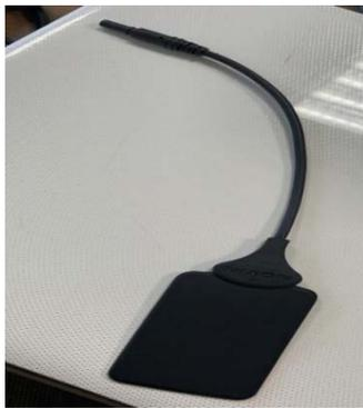
**Figure 2.** Rubber electrode
