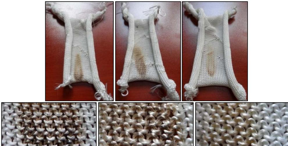
Figure 8. Pictures taken after the burning test of completely glass yarn GG/GG fabric knitted at 4 cam settings.
