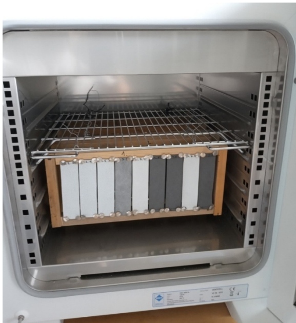
Figure 4. Test specimens attached in wooden frames, placed in drying oven.
