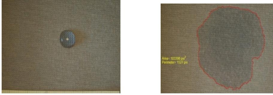
**Figure 10.** Kinetics of spreading of water drops on polyester fabric: (a) time 2 s, (b) time 120 s and calculated contour.
