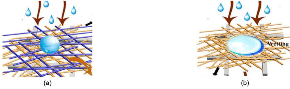
Figure 7. Water droplets on the surface of (a) hydrophobic fiber layers, (b) hydrophilic fiber layers (modified from [20]).
