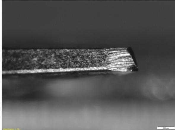
**Figure 3.** Reground tooth tip of a clothing, top view.
