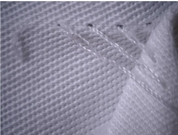
Figure 6. Mechanically damaged cotton fabric - loose pocket, suitable for repair, enlarged 15x.
