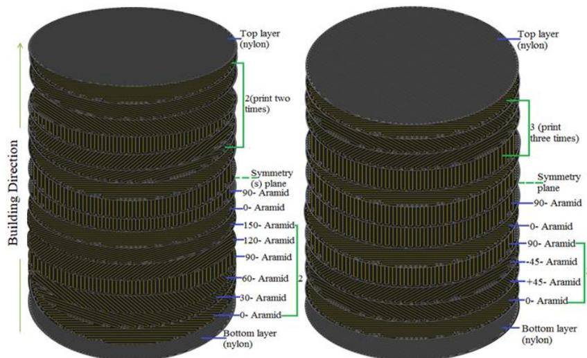
**Figure 7.** Example of material arrangement and printing order of aramid layers- at filling angles [(0/30/60/90/120/150)2/0/90]<sub>s</sub> and [(0/+45/90/-45)3/0/90]<sub>s</sub>, generated by Eiger.io of [56].
