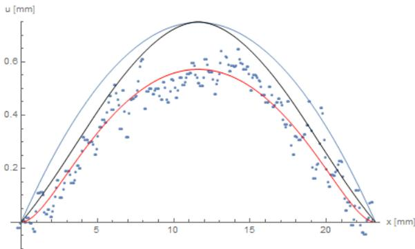
**Figure 9.** A comparison of the measured deflection of the fabric skin, loaded by 100 kPa (blue dots). The theoretical curve, derived from the equation, is shown in red. The interpolated simulation data is represented in black and a theoretical curve, which neglects the bending stiffness, is illustrated in blue.
