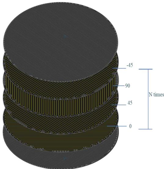
**Figure 2.** An example of material arrangement and printing order of polymers at filling angle  $(0/+45/90/-45)_N$ , generated from Eiger.io.
