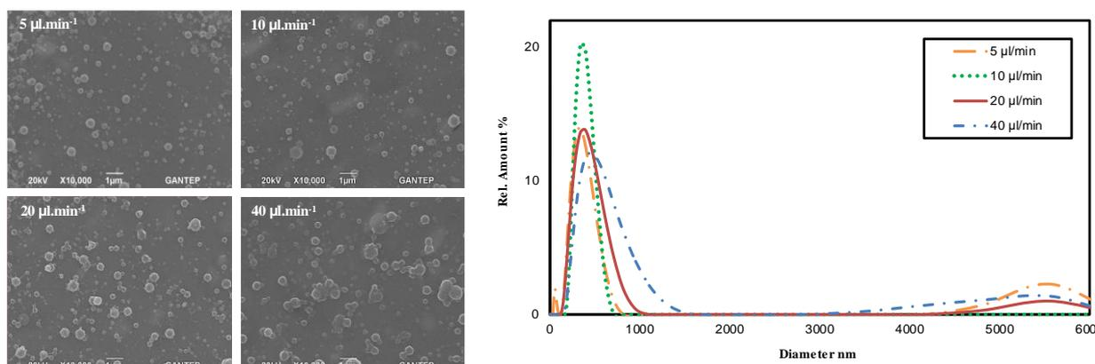
Figure 1. SEM images and size distributions (intensity) of nanocapsules at various total flow rates.
