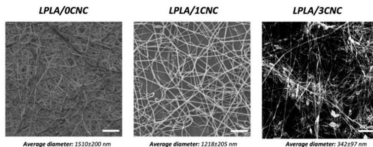
**Figure 3.** Electrospun bio-nanocomposite webs of LPLA having different CNC content levels.
