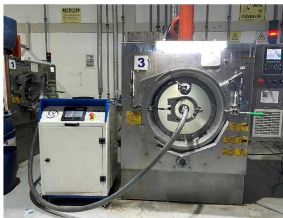
Figure 1. Foam generator and washing machine used in the study.
