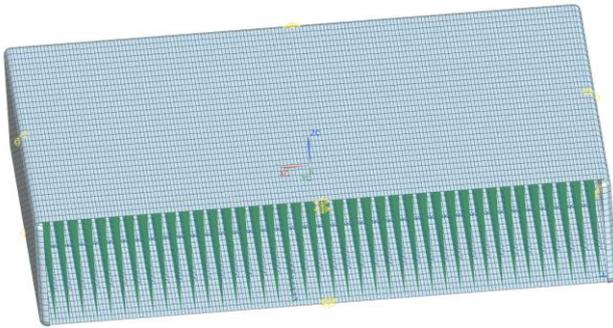
**Figure 5.** A section of the simulation model of the 3D distance panel. The mesh on the skins is created in such a way that four elements are placed after warp, which ensures an accurate representation of skin deflection. The green lines represent pile yarns, while the blue crosses represent suppressed displacements.
