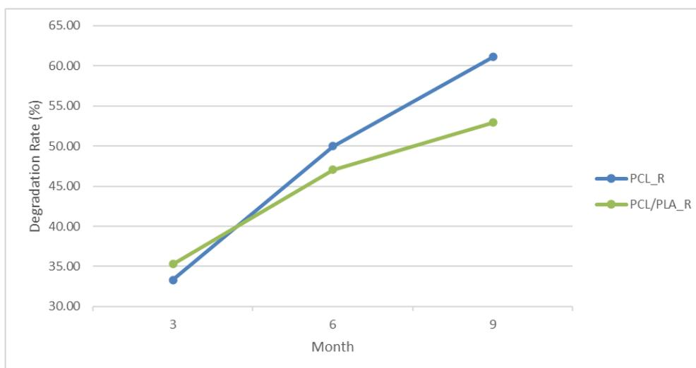
**Figure 1.** Biodegradation rates of PCL\_R and PCL/PLA\_R scaffolds.
