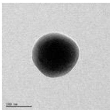
Figure 6. TEM image of nanocapsules at 5/5  $\mu\text{l}.\text{min}^{-1}$  flow rate ratio and 26/22 G needle.
