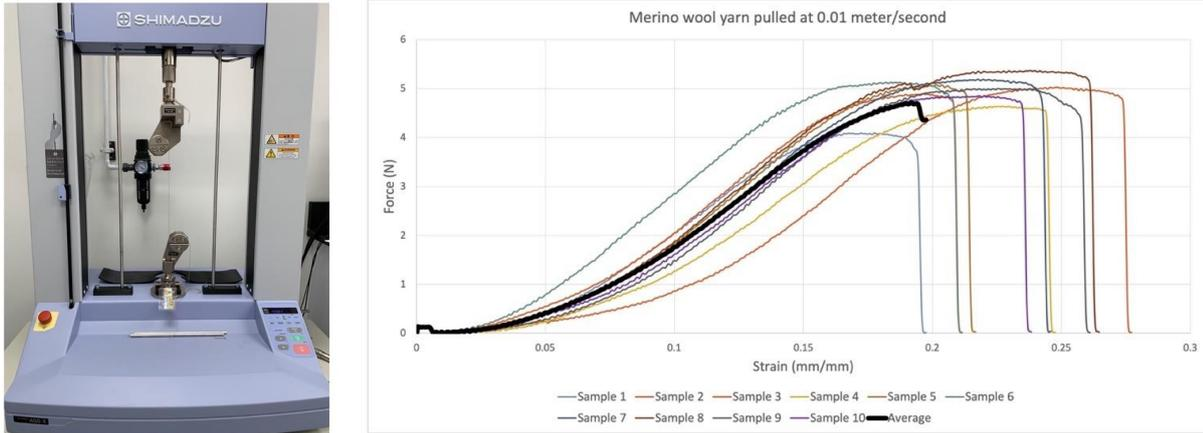
**Figure 4.** (Left) Merino wool yarn loaded in capstan grips on the Shimadzu load frame. (Right) Force vs. strain data for 10 samples of Merino wool yarn.
