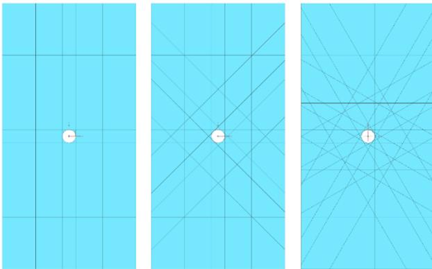
**Figure 2.** CAD model of FOF laminate layouts:  $[0/90]$ ,  $[0/45]$  and  $[0/30/60]$ .
