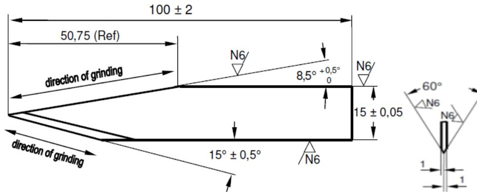
Figure 3. Geometry of the test blade P1/B (dimensions in mm) [52].
