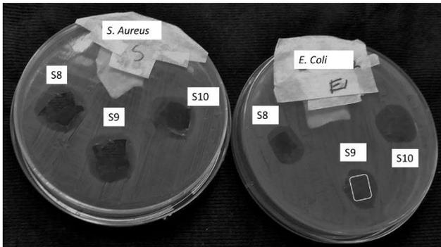
**Figure 3.** Antibacterial properties with Zone of inhibition.
