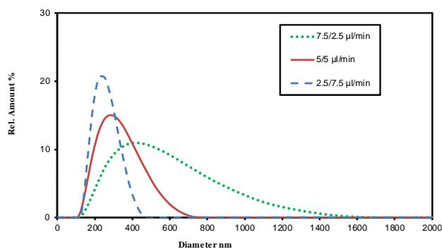
Figure 3. Size distributions (intensity) of nanocapsules at various core/shell flow rate ratios.
