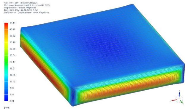
Figure 6. Displacements of pressure loaded fabric panel.
