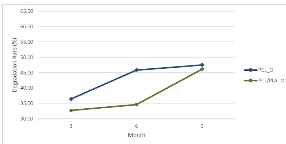
**Figure 2.** Biodegradation rates of PCL\_O and PCL/PLA\_O scaffolds.
