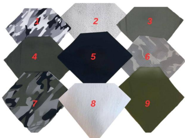
Figure 1. Investigated camouflage fabric samples: Sample №1 – Rip-Stop "Comfort", khaki color; Sample №2 – Rip-Stop "Comfort", dark blue color; Sample №3 – Rip-Stop "TC"; Sample №4 – "Olive"; Sample №5 – "Khaki"; Sample №6 – "Defensa"; Sample №7 – "White Night". Investigated blended hemp fabric samples: Sample №8 – Blended hemp fabric, broken twill weave 2/2; Sample №9 – Blended hemp fabric, plain weave 1/1.
