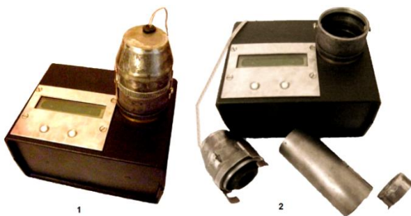
Figure 6. Device appearance: 1) in operating condition; 2) with the measuring chamber removed.
