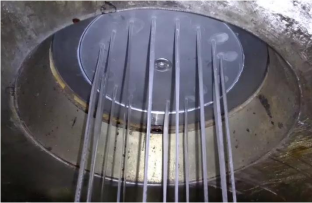
Figure 1. Spinneret outlet in detail view during production of liquid filled hollow fibres.
